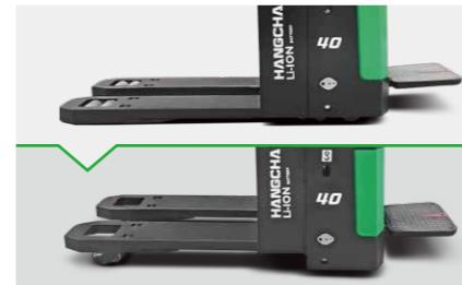
The unique floating suspension system enable the driving wheel to contact the ground all the time. The booster cylinder equipped can adjust the road holding of the driving wheel along with the lifted loads to prevent slippage and ensure good stability of the forklift.
