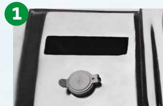
The battery box cover is designed with an air spring to allow the cover to be opened more easily.
