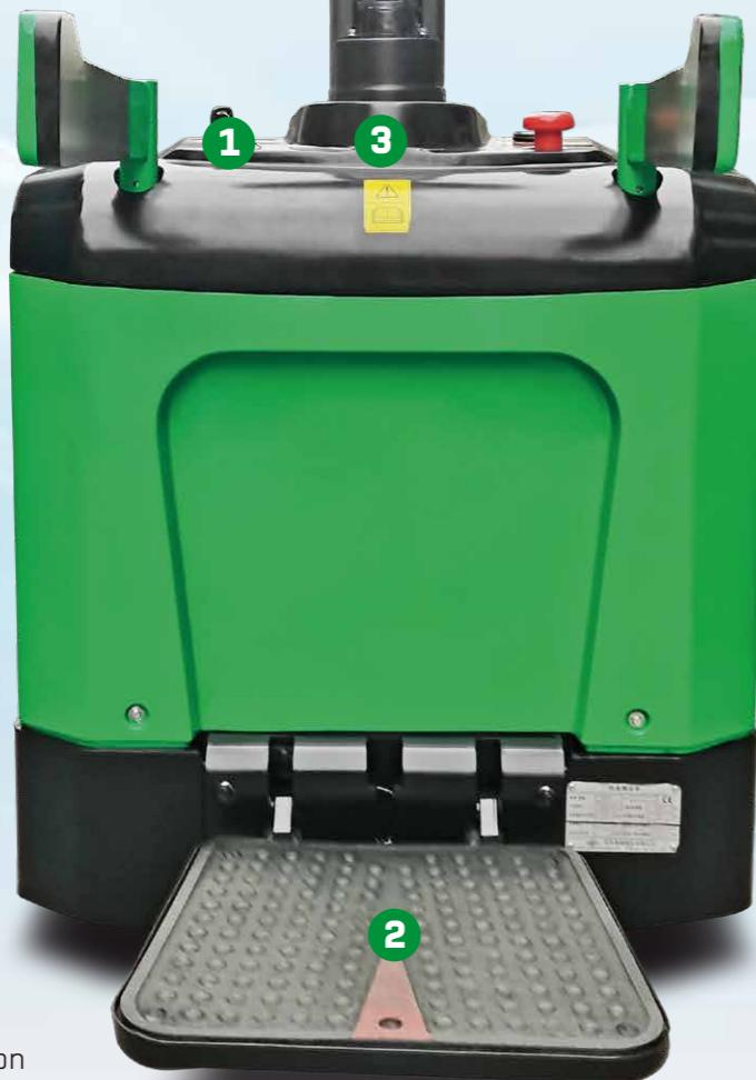
Designed with shock-absorbing function, the pedal can greatly improve the ride comfort and alleviate the operator's fatigue due to long-time driving.
